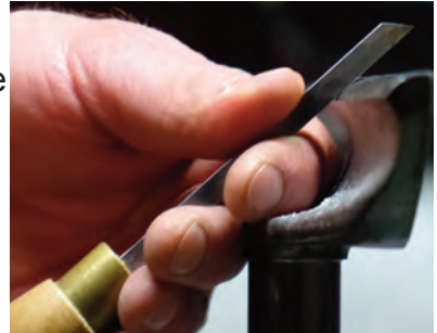
Starting approach angle for the beading tool making the rings
