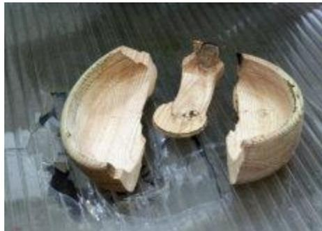
Francois brought in this lesson to us all as to what can happen - and how safety concerns should be paramount! The gouge caught on a knot with the lathe turning at 2500 rpm, spinning off and hitting the roof with dramatic results.
