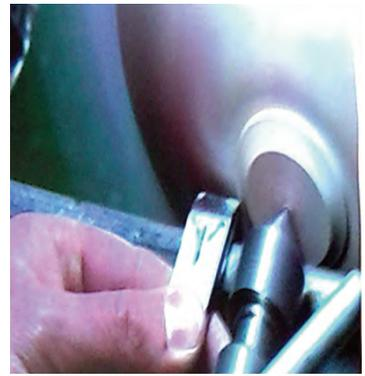
L to R: Simple jig for holding partly finished bowl. Positioning bowl on the jig. Held in place by the tailstock centre, the foot is cleaned up
