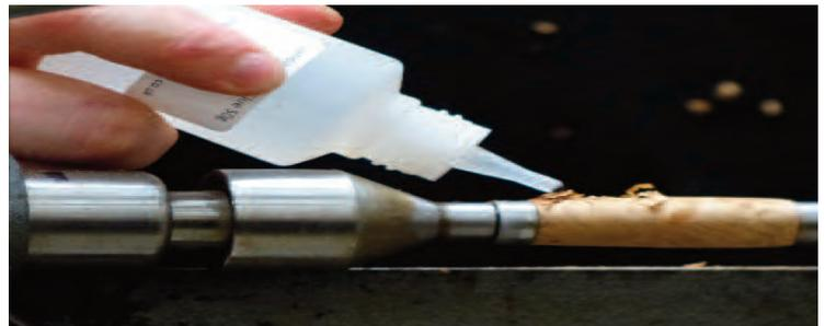
*Applying super glue to sawdust to fill a gap*
