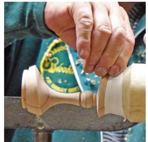
Plastic tape ensures that the jam joint cannot come apart
