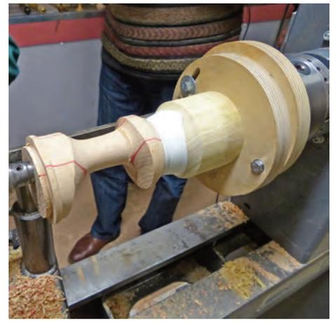
*The off-centre jig with the adjustment bolts*
