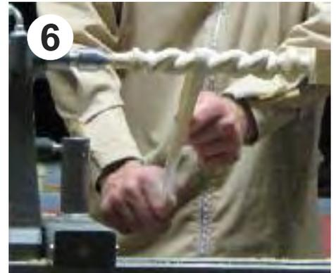
1: finished spiral with roughly shaped copy. 2: the tapered shaft is marked with spiral positions. 3: Richard starts by cutting on the lines with a tenon saw. 4: a small Microplane is used to widen the saw cuts. 5: the wider Microplane cuts deeper and wider to get near to the final shape. 6: The final touches (apart from finishing). A band of abrasive is used for smoothing all over.
