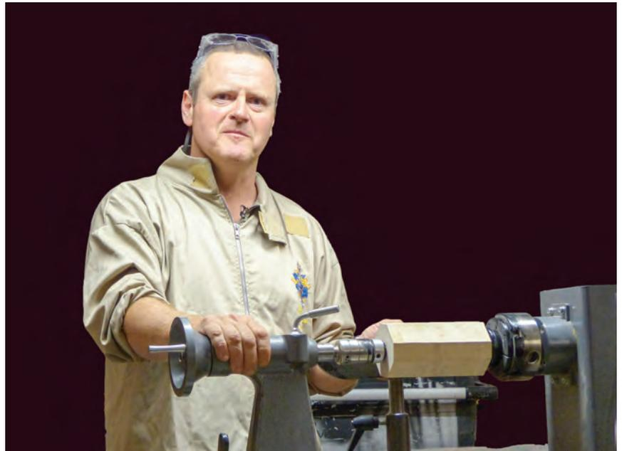
*Above: rippled sycamore ready to be converted into a Crushgrind mill. The corners have been trimmed to form an easy-to-rough-down octagon. Below: Les takes to his sketching board to explain the mechanism of the Crushgrind*
