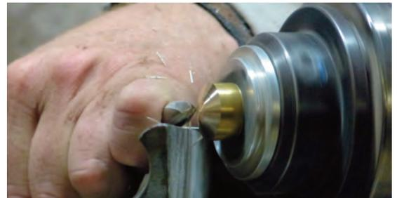
Shaping the top with a spindle gouge
