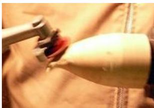
The lid was given a final fit to the base by sanding with 320 and 400 grit (turn the sanding strip over to give a final burnish). The spigot on the base was removed using a jam chuck and the piece should be finished off with 3 coats of lacquer.
