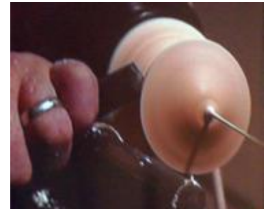
Using a skew to produce a hollow base on the goblet
