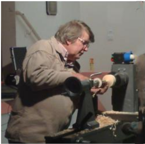
Tony supports the fine stem while turning one-handed
