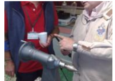
Tony points out the convex grind on his skew ensuring some part of it touches the wood at all times to prevent snatching
