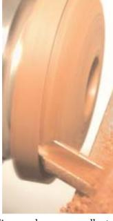
To finish the base power sanding produces an excellent surface. Whether by hand or under power on hardwoods, I always end up with 1500 grit Webrax to give a burnished finish.
