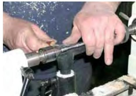
*Metalwork: turning a lace bobbin in aluminium*
