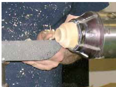
Box lid: showing how to cut the male thread
