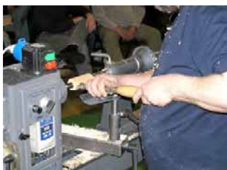
Texturing: making a pattern on a parallel spindle
