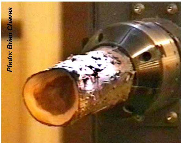
Just starting: the yew branch is mounted and hollow started
