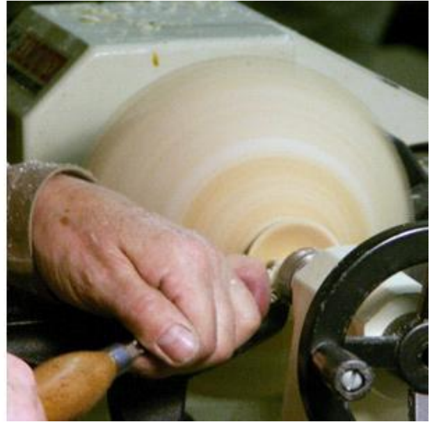
Cleaning the bottom
