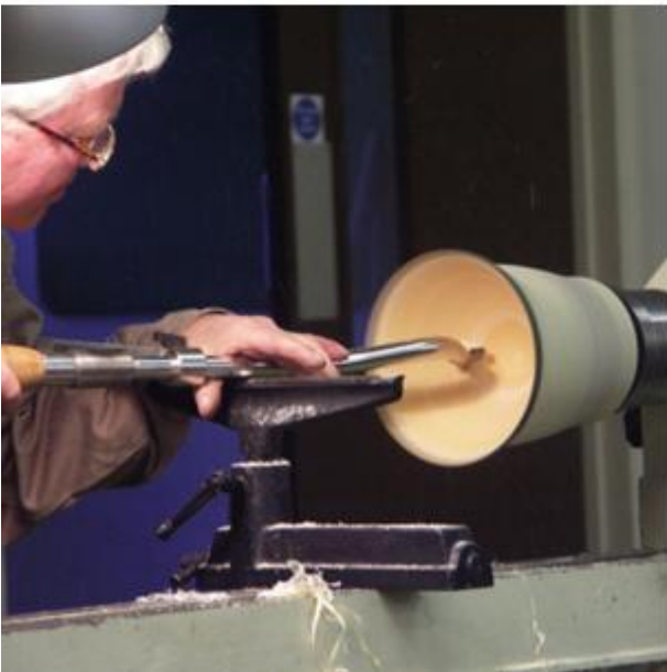
Shear scraping the inside
