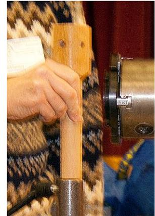
When mounting a uneven blank on the lathe Jeff has turned his own version of the Elio drive which allows for the wood to be mounted when it you don't necessarily want the blank to be parallel to the chuck or is uneven. This is made with wood and chipboard screws to the length necessary and is more secure than a simple screw chuck.
