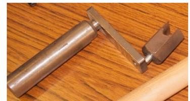
Although Jeff has purchased a number of hollowing tools he finds the most successful ones (apart from the Rolly Munro, which he has never owned) are the ones he has made himself, ground out of masonry drills and caps out of mild steel.
