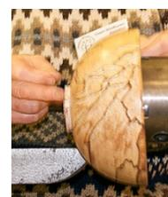
A shear scraper is made from a tyre lever filed down – the tyre lever is strong steel and not brittle, he remarked that it is not a good idea to use a filed down file as they can break with disastrous consequences.
