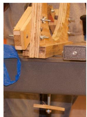
Gordon also uses an extension for sanding inside hollow vessels, but in this case it is a drill extension with a sanding wheel on the end, this can be replaced with a sanding disc for the bottom of a vase.
