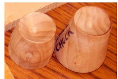
Jeff reminded us that we can use a rubber mat on the faceplate or chuck and a flat piece of wood on the tail stock to hold a piece in place or to use as a clamp.
