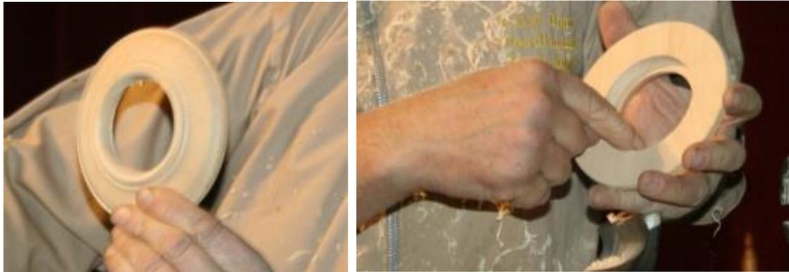
Gary followed this with his main demonstration of a Mexican Rosewood (Bocote) box with a Corian inlay in the lid. He started mounting the 2½” blank with the corners removed between steb centre and tail stock.
