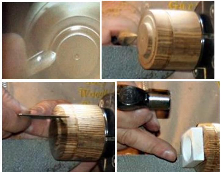
The wood and Corian were then turned to give the impression that the Corian was inserted into the wood (this only works with a curved surface). Remember to make sure you are careful when turning Corian which blunts the tools fast and is very messy (a mask should be worn).
