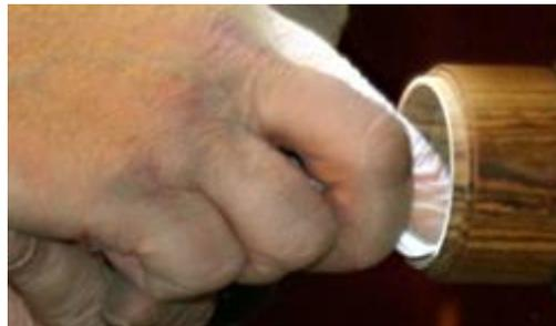
The base was then removed from the chuck, reversed and mounted on a jam chuck in order to finish off the bottom of the box. Despite the quality of the finished article Gary said he finds that boxes don't sell very well and this would usually only only sell for £40 up to a maximum of £55-£60
