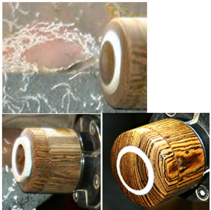
When complete the lid was removed – *if the lid is too tight to remove try using a block of softer wood to tap it off*) and the inside of the box finished. *If using a box scraper remember to set the tool rest higher then tip the tool slightly to go down the side and very gently across the bottom*
