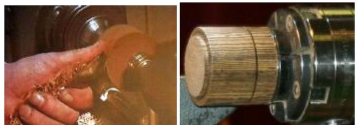
The lid was then cleaned up with a spindle gouge – either getting the bevel and cutting in or going into the centre and drag it back. It was then cleaned up with a ¼” skew or a box scraper, keeping the handle low and scraping across .
