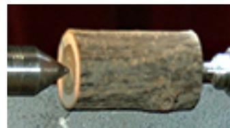
The log was mounted between steb centre and tailstock and skew was used to flatten the end. The length was marked and the size was stepped down with a skew – rocking it from side to side
