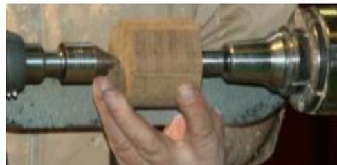
The blank was roughed with a roughing gouge – with the handle dropped to go in at an angle and Gary uses his thumb over the top of the gouge to deflect the shavings they are removed. He turned a 1/8” spigot on both ends. The point where the lid was to be was marked then the blank was re-mounted in the chuck at the lid end and parted off.
