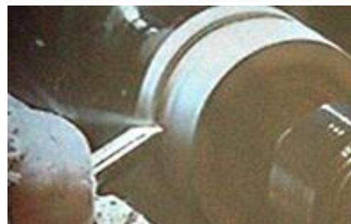
The shape was made with a skew, with the tool rest low and the skew handle dropped and lifted up. A ¼ " spindle gouge was used to soften the bead.
