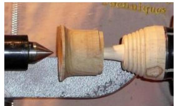
The inside of the bell was then turned so that the funnel fitted exactly in place and a 12mm hole was drilled through and then tapped to create the thread for the handle. The fit of the funnel into the bell was checked, lining up the grain and using superglue the funnel was fitted into place.
