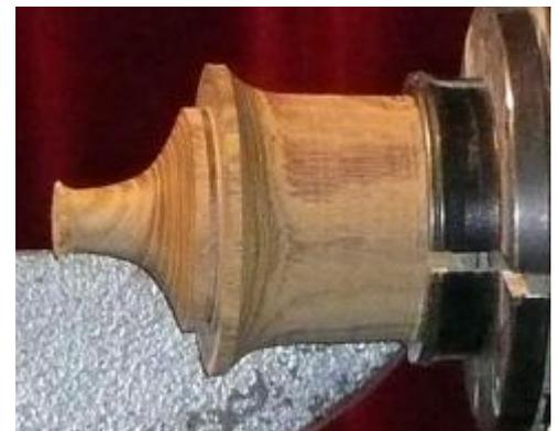
A cylinder was rouged down to 58mm and Gary used a skew chisel to make the funnel shape.
