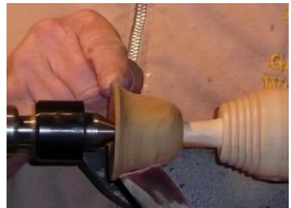
The handle was turned in ebony - an ideal wood for thread chasing. Gary showed us his 'scratcher' which is a piece of wood with metal points to check the length and with all the dimensions of the handle drawn on - useful for repeating pieces.
