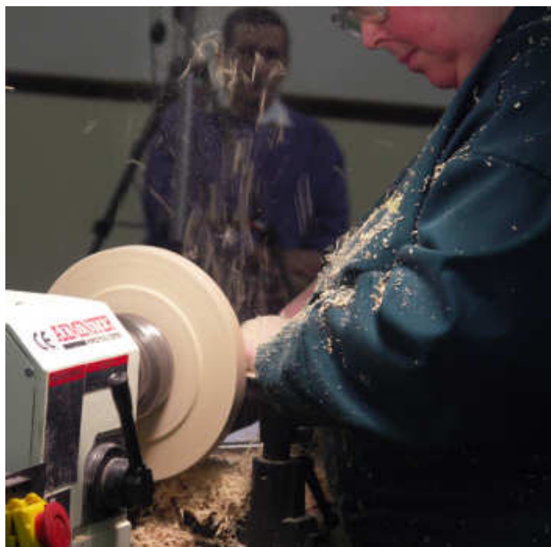
Truing the surface
