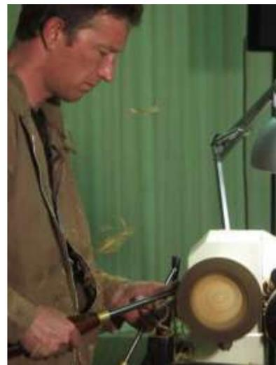
Once the item had been roughed out, reversed chucked and sanded on the outside and flamed using methylated spirit to raise the grain and finally sanded with 240 grit paper, he started to demonstrate his colouring method using Chestnut spirit stains, explaining that the whole concept of the process is an art form rather than a science, open to experiment and ones own flare, likes and dislikes.
