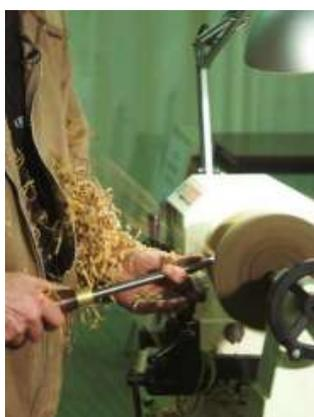
Finishing cut with the long grind bowl
