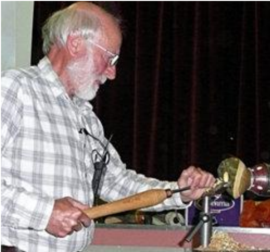
Peter holds the gouge down hard on the rest and moves to a larger gouge later on.
