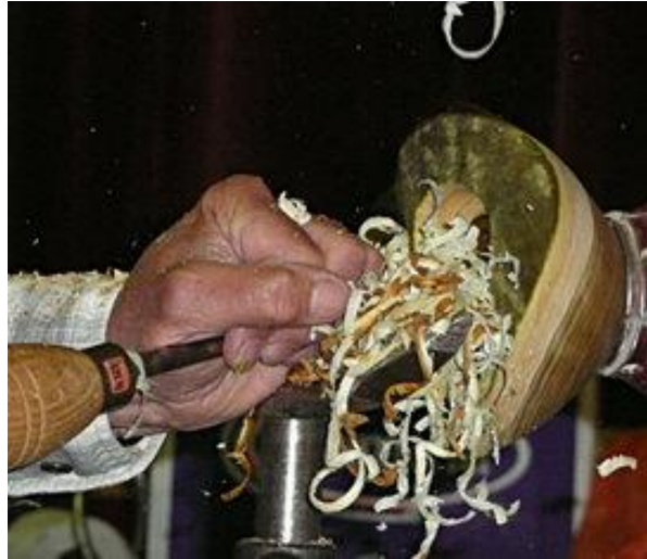
Peter holds the gouge down hard on the rest and moves to a larger gouge later on.
