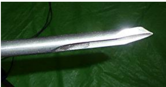
He uses a gouge with an Ellsworth cut - very swept back wings to get the blend into existing curve. It is better to take big cuts for the last few cuts so the wood wall doesn't vibrate too much. Using a swept back Ellsworth cut gouge he finishes the centre starting at the middle and pulling outwards with gouge at 10 o'clock, then he works from the outside in - gouge at 2 o'clock.
