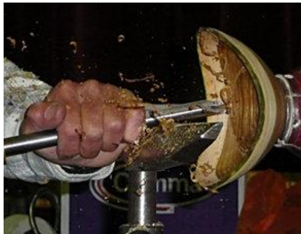
Peter holds the gouge down hard on the rest and moves to a larger gouge later on.
