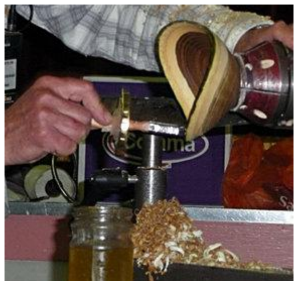
After a fine cut at the end apply a coat of melamine sealer and leave to dry.
