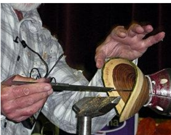
Keep stopping to check – use the calipers to measure the depth and check on the outside to make sure you don't go in too deep – when you see a patch of light at the bottom you know you've gone too far! The wall thickness needs to be the same throughout or the wood will dry unevenly and crack.
