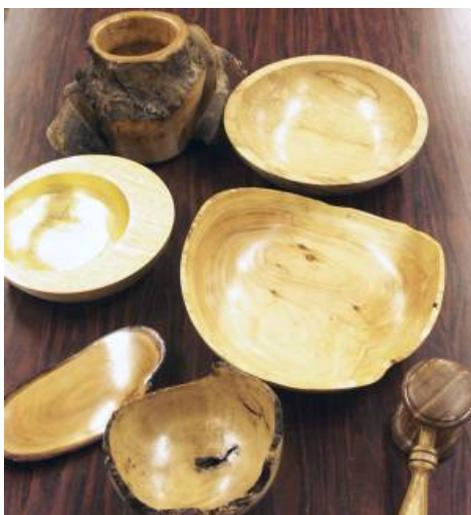
Finally Roy showed us how he mounts a wooden spigot inside the bowl with a bead of hot melt glue so that a new chuck recess can be turned on the base ready for finish turning. The outside of the bowl is then finish using a smaller bowl gouge which produces smaller cutting forces. Finally the inside is turned to produce an even wall thickness of 10mm. To finish the bowl Roy would normally use an oil finish such as Danish Oil.
