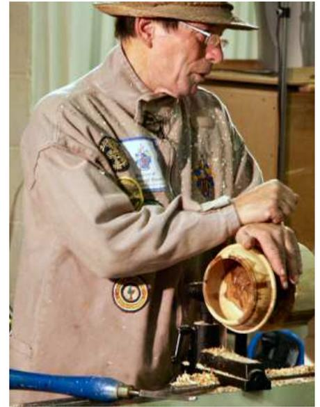
Having measured and marked the depth of the bowl on the outside of the blank he then turned the bowl outside to about 1/8" thickness. The based had been left about twice the side's thickness to give extra weight and balance to the base. He would normally have sanded the bowl after cutting but explained that under demonstration conditions and without the air filter system on, did not want to create too much dust.
