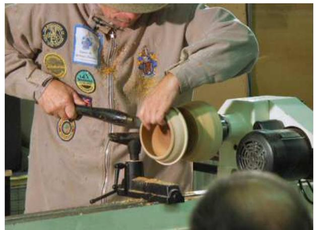
The bowl was completed with texturing and 'painting', with a vinegar/ wire wool mixture. After parting off the bowl the remaining wood was used as a jam chuck in reversing the bowl to clean up the foot. Stuart would then normally microwave the bowl for final drying.
