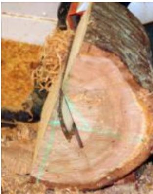
¼ sawn log – removing the pith from the centre of the log
