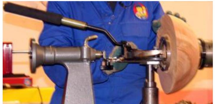
The system will produce bowls up to about 16" diameter. The Woodcut system has a set curve so the bowls will always be the same shape. The McNaughton system can be adjusted to produce a different shape of bowl but Jeff found it very much a trial and error process to get it working successfully and there seems to be more danger of damaging the lathe in the process.
