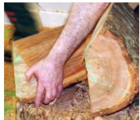
When Tim cuts logs that aren't going to be used immediately he wraps the ends with plastic bags, sealed with tape to prevent the ends drying out.
