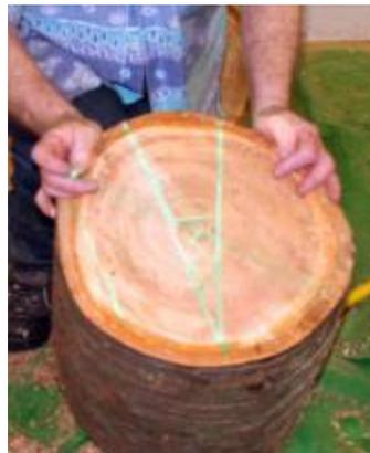
Alternative way to remove the pith to produce 2 large blanks
