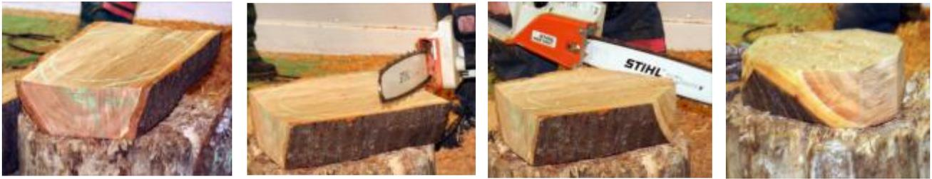
He demonstrated options for cutting the log to produce different sizes of blank and removing the central pith:
