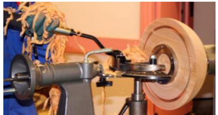
When the first bowl is removed the centre of the bowl remaining on the chuck is cleaned up and the blank is remounted with the faceplate in order to cut a new spigot. The spigot should be substantial as it can easily be ripped off.
