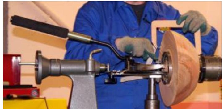
A template is provided to help you set up the mechanism correctly. The cut is on the centre line and it is important to get it precisely set up. Cutting support is provided by the tool post and tail stock
