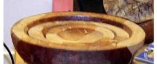
Jeff started by mounting a faceplate onto the blank and turning it to a bowl shape with a spigot. It was then turned round and held in the chuck, the faceplate was left in place as it would be required later on.
