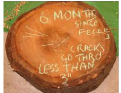
Tim marked out the log to indicate how best to remove the pith in the centre of the log – if left in the wood will split from that point.
