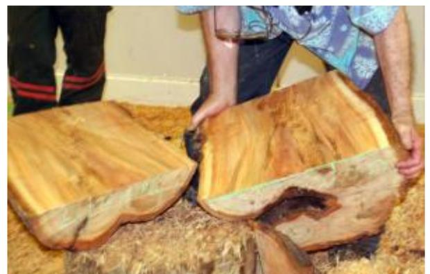
In the second part of the evening we had a demonstration by Jeff Cordery of his bowl saver. This is a way of cutting more than one bowl out of a blank, making a nested set. In this case he used the blank previously cut by Tim. Whilst it is possible to work with dried wood with the bowl saver it is much harder work and will take much longer so it is preferable to use wet wood.
