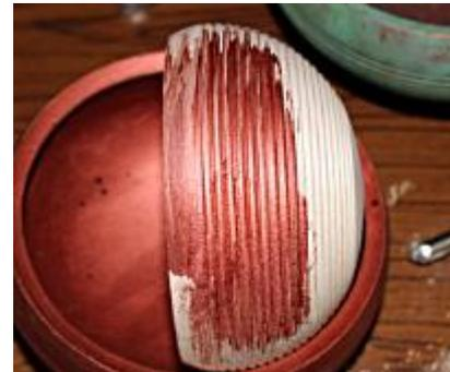
Mark showed us how he coloured the bowl, initially using a toothbrush to apply 2 coats of bronze paste, which he finds works better than sprays. He then produced 'one he had made earlier' where the paste had been applied to the whole surface.
