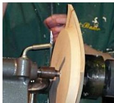
He told us to slow down if necessary when going into the centre, removing as much of the centre as possible with the piece still supported by the tailstock. Drop the handle arcing toward the centre – use a pull cut for better surface and a scraper for blending the section.
