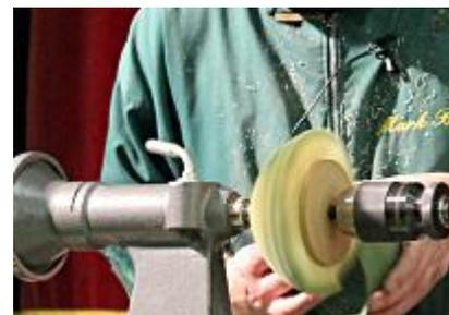
A dome drill brush mounted in a jacobs chuck on the lathe was used to unevenly brush off the verdigris, at a slow speed with a gentle touch, creating highlights on the surface – this will take around 15 minutes. This finish is not food safe.
