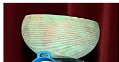
The bowl was turned with the widest point 1/3<sup>rd</sup> of the way down from the top. Mark smoothed the outside with a scraper which has a negative rake with the tool held horizontally to the work. He sharpens the scraper with a diamond file just on the underneath edge and only re-grinds the top when the negative rake has worn away.
