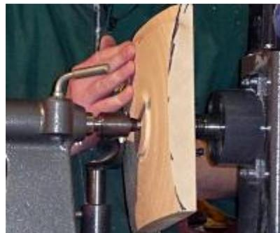
He removed the ridges, dropping the handle of the bowl gouge and using it as a shear scraper. He spoke about sanding – always going one grade of abrasive coarser than you think you need. He uses sanding pads and said he would finish off the wing tips by hand – not while the piece is spinning if you want to keep your fingertips!
