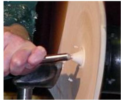
Once the inside is finished Mark turned the piece round to finish off the base – this would be smooth and rounded. He used a turned block as a support padded with kitchen paper and again used the tailstock for support. If possible this should be wider, perhaps a revolving step centre or failing that use blue-tak and a washer on the tailstock to prevent the pointed centre going through. He blended it in with a scraper and then removed it and took off the final 'pip' by hand
