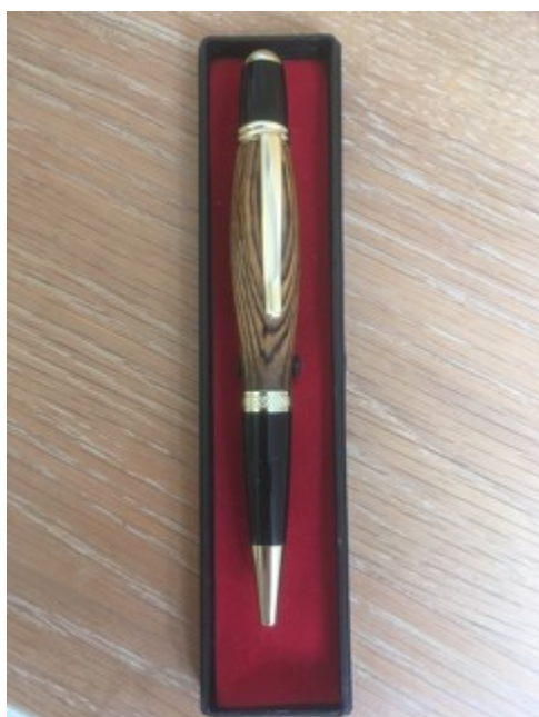
Pen made from Bocote wood and finished with melamine lacquer
