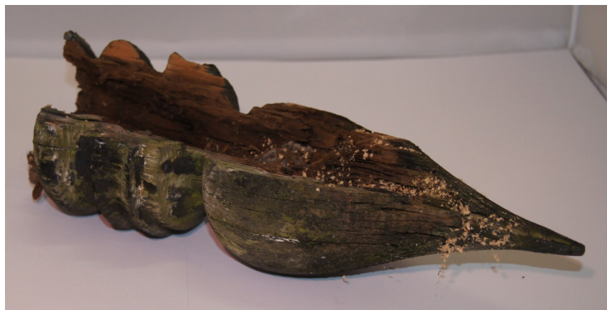
David Curnow was tasked by someone to reproduce the object below which has seen better days. It is a large finial which sits at the apex of a porch. A great copy finished with sanding sealer.
