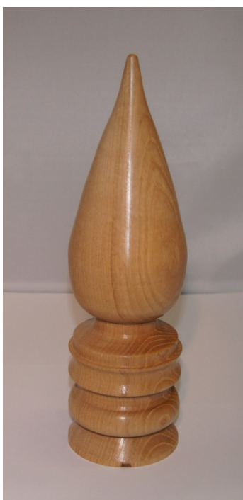
David Curnow was tasked by someone to reproduce the object below which has seen better days. It is a large finial which sits at the apex of a porch. A great copy finished with sanding sealer.
